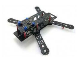
With rubber damper to decrease vibration during flight.
