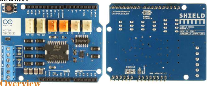
The Arduino Motor Shield is based on the L298 (datasheet), which is a dual full-bridge driver designed to drive inductive loads such as relays, solenoids, DC and stepping motors. It lets you drive two DC motors with your Arduino board, controlling the speed and direction of each one independently. You can also
