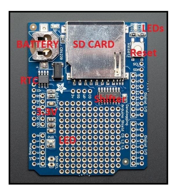
The datalogger shield has a few things to make it an excellent way to track data
