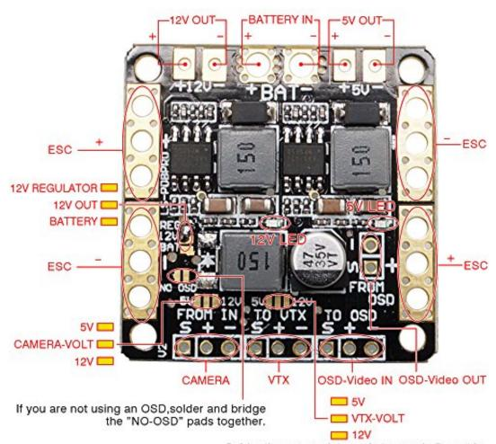
Solder the appropriate pads to supply 5v or 12v to the CCD board camera and video transmitter.
